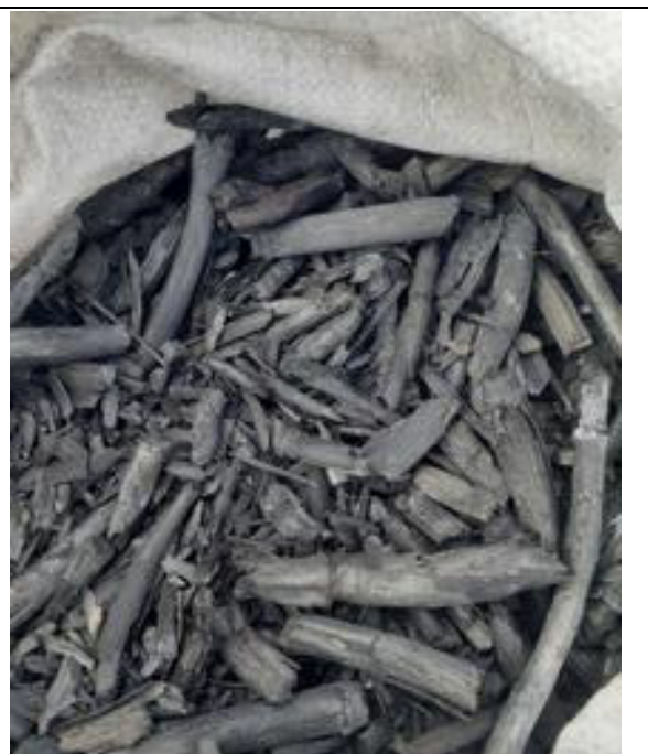
Very good quality char from maize stalks in bag 1: lightweight, brittle, easy to crush to powder
